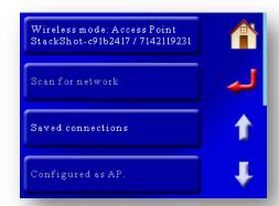
If you do not see "Wireless mode: Access point", then simply press that button to switch the controller to an access point.
