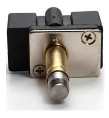
3. Place the black portion of the valve with the wires coming out of it over the slug and adjust its position so that it covers the metal plate. The smooth surface should mate up with the valve body. The wires should be away from the valve body.
