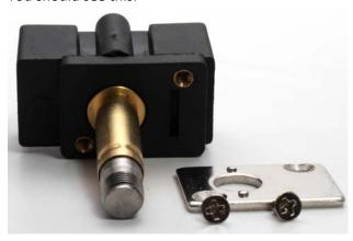
5. Pull on the brass portion of the valve to remove the plunger. The silver metal end with the spring may fall out of the brass (no worries).
