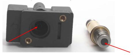
7. The valve is now cleaned! Time for reassembling.
